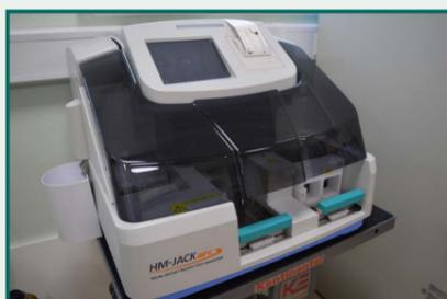
Figure 2 - HMJACKarc Analyser
