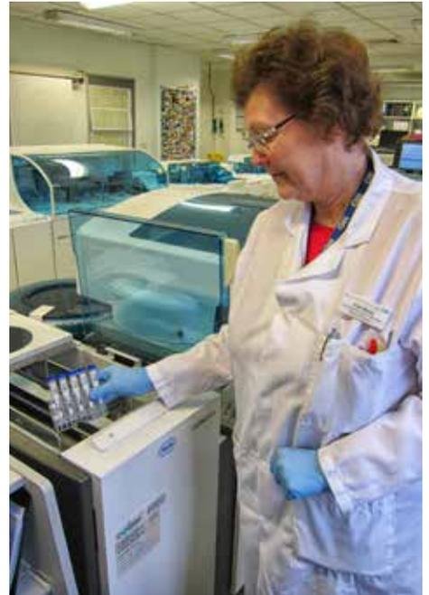
Pamela Bowe loads BÜHLMANN fCAL<sup>®</sup> turbo faecal calprotectin tests onto the Roche cobas<sup>®</sup> 6000 c501 analyser
